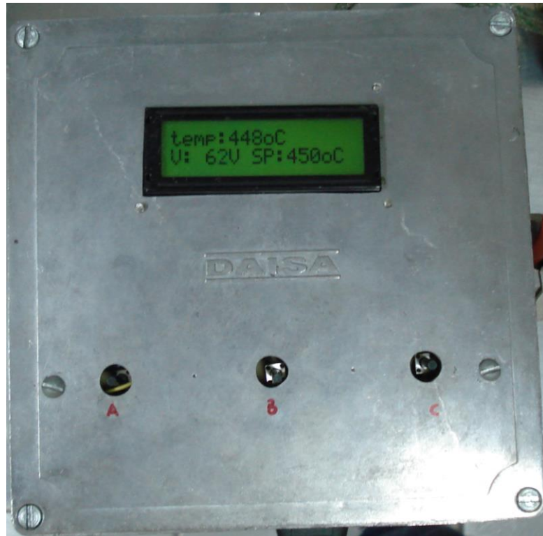
Fig. 21 Photo of the case of the power controller with hot filament
