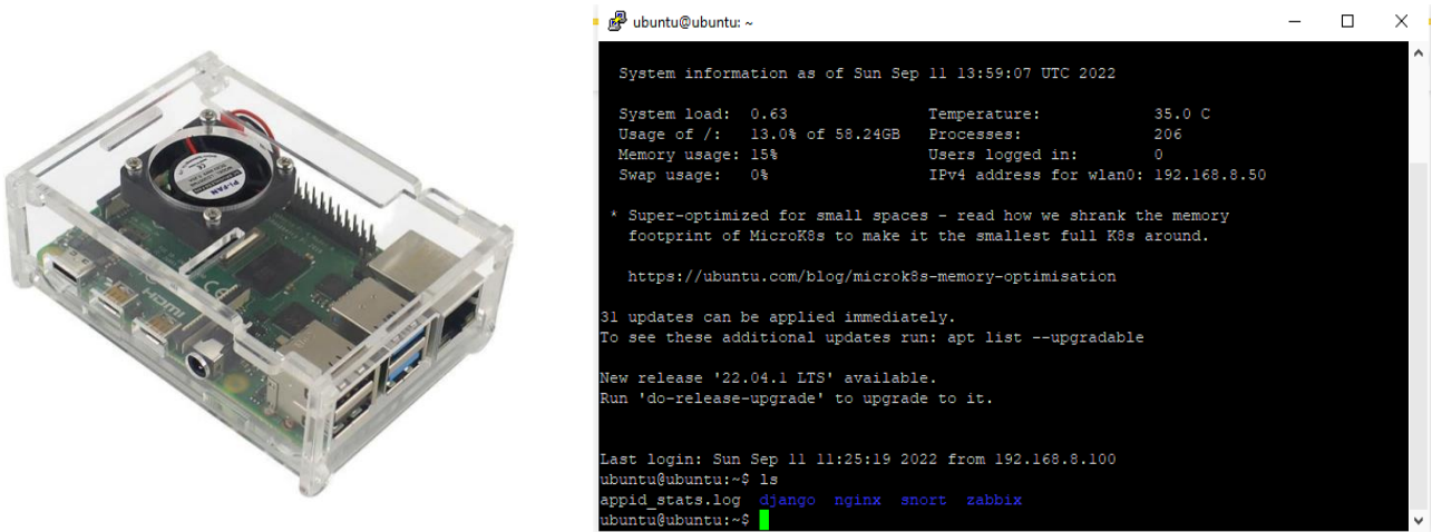
Fig. 3 Raspberry Pi4 and attempt to harvest data from snort
