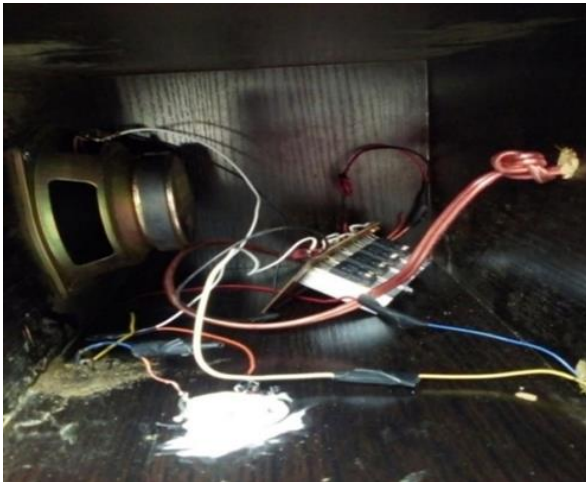
Fig. 5 Guming the component to the casing
